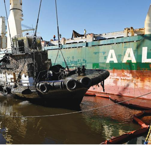
AAL Shipping salvaged two tugs in Tasmania. The tugs sank in January after being hit by a cement carrier while berthed. A seven-month planning operation ended when the AAL Melbourne departed from Devonport with the wrecks of the York Cove and Campbell Cove on board. The tugs were welded to bespoke cradles on the deck of the AAL Melbourne for the voyage to Brisbane, for scrapping.
