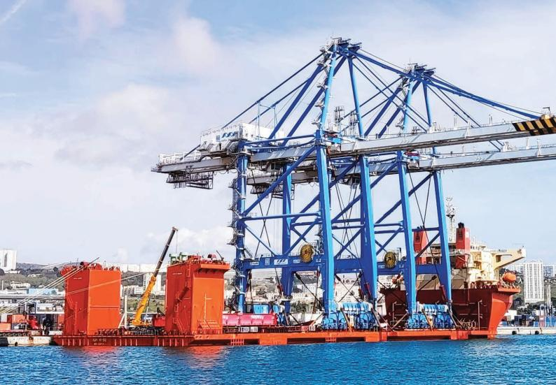
Ceva worked with Italian transport engineering and heavy lift specialist Fagiori to relocate two 1,700 tonne ship to shore cranes from Malta to Marseille, France.
